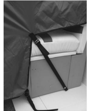
The initial assembly of your Pontoon Enclosure is now complete. Note that the windows and doorway can be rolled up and out of the way when desired - held in place with Hook & Loop straps.
