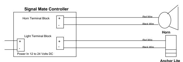
Signal Mate is capable of 20 amp (max) fuses for both horn & anchor Light.
