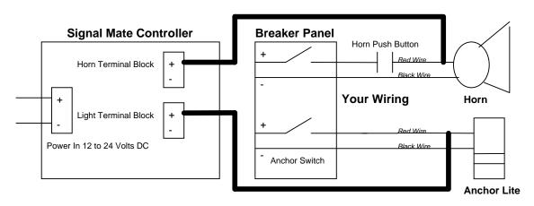
Just add 2 wires one to the horn side of push button the second to the anchor side of breaker switch.
